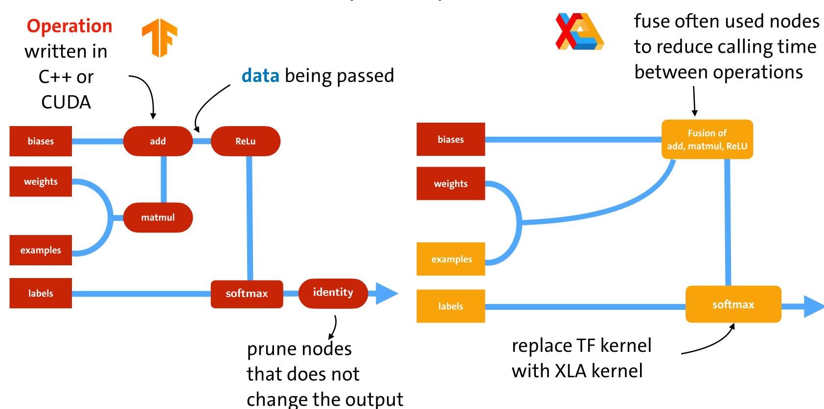
AOT compile of a graph means to compile it statically into self-contained libraries (header-object pair). The models becomes a series of C++ compute kernels.
