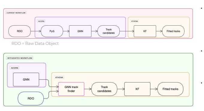
Previously, Acorn used to build tracks, which were passed back into Athena for fitting Now, models trained in Acorn, translated to Onnx and TorchScript Loaded into Athena Component (c++) as part of tracking chain
