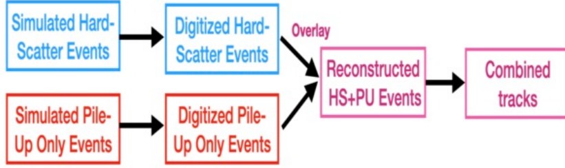
Figure 1: Diagram of the MC overlay process, where simulated pile-up collisions are digitized separately and then combined, followed by the reconstruction algorithm.
