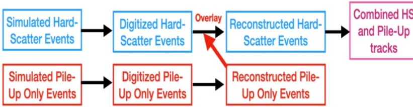
Figure 2: In the track overlay method, pre-reconstructed pile-up tracks are overlaid onto HS digitized events, followed by the reconstruction process.
