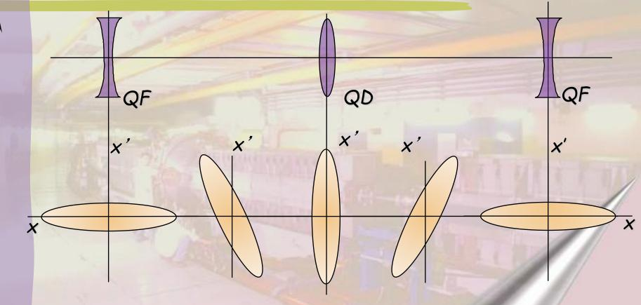
✓ For each point along the machine the ellipse has a particular orientation, but the area remains the same
