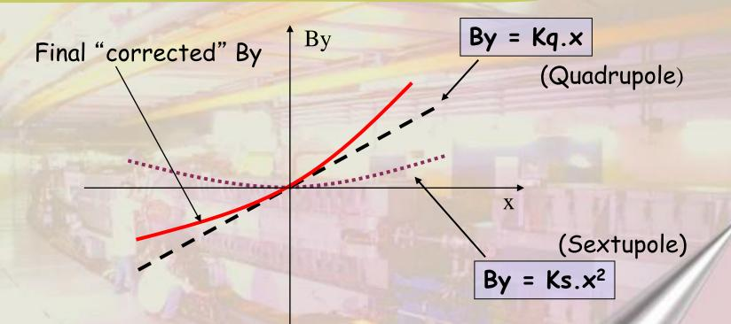
Vertical magnetic field versus horizontal displacement in a quadrupole and a sextupole.
