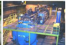
Cold boxes from world wide leading industries (>100t, Heat exchangers, expansion turbines, valves, controls)
