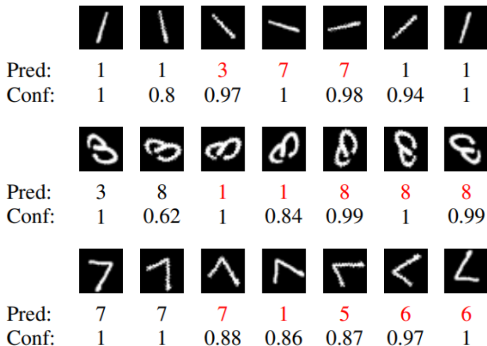
Fig. 5: Predictions received from a LeNet network trained on MNIST's handwritten digits from 0 to 9 and evaluated on different rotations of test samples.
