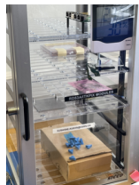
Humidity-controlled environments with dry-air desiccators(CERN)
