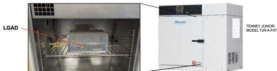
Humidity and temperature are measured inside the metal box (BNL)
