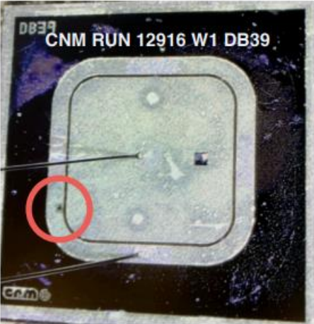
burn mark in the CNM sensor after ATLAS TB in 2018 after the test beam – dimensions are few tens μm (crater photo taken by CNM)
