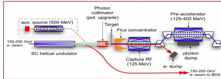
Electron driven positron source
