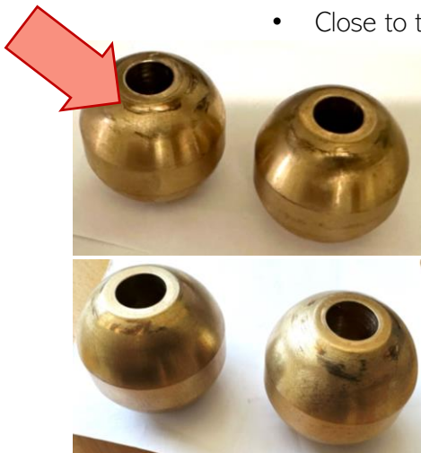
The contact area measured from the wear on the bearings
