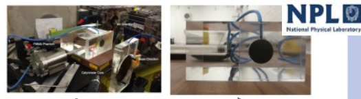
Figure 5. (a) The test-stand at the CLEAR facility, with the calorimeter, ion chamber and monitor chamber placed along the beam line with the beam travelling from right to left. The calorimeter core can be seen at the end of the PMMA sleeve (b). This shows the front surface of the custom PMMA phantom with beam monitor insert placed to the right of the calorimeter sleeve. The PMMA build-up blocks, used to ensure the reference depth of the detectors was at 8 cm, are not included in the photographs.
