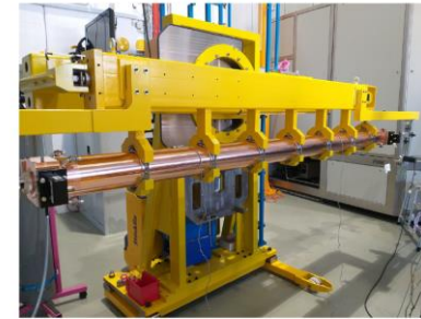
Fig. 3. HG1 structure on the holder during bead pull test with a wire passing through beam pipe.
