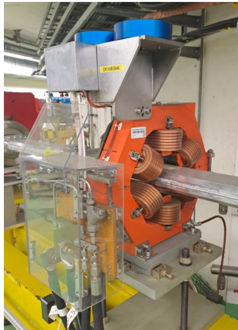
Renewed quads and sextupoles with large aperture
