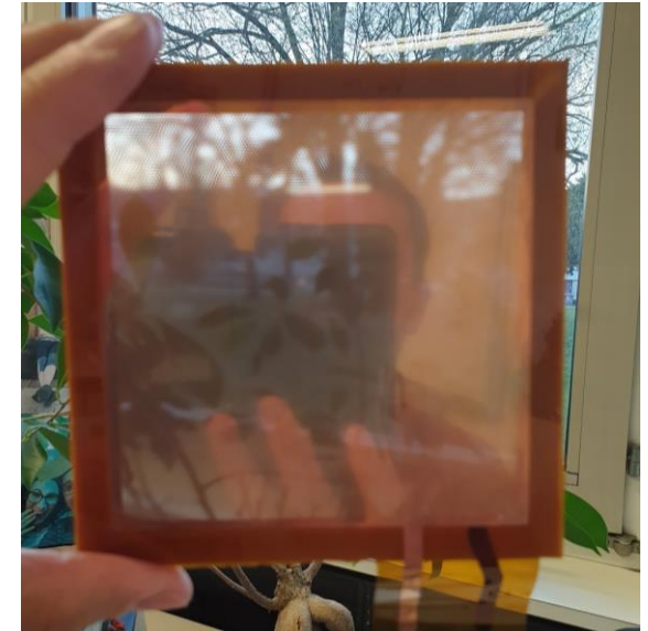
Gas electron multiplier (GEM)
