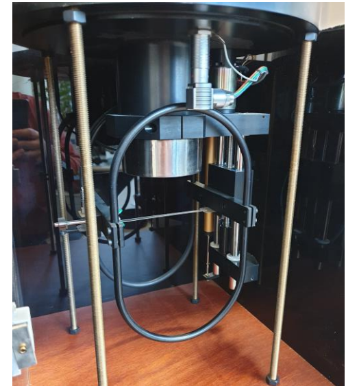
Finger scintillator scanner (FISC)
