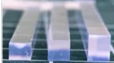
38 m 2 of LYSO Crystals in Barrel Timing Layer
