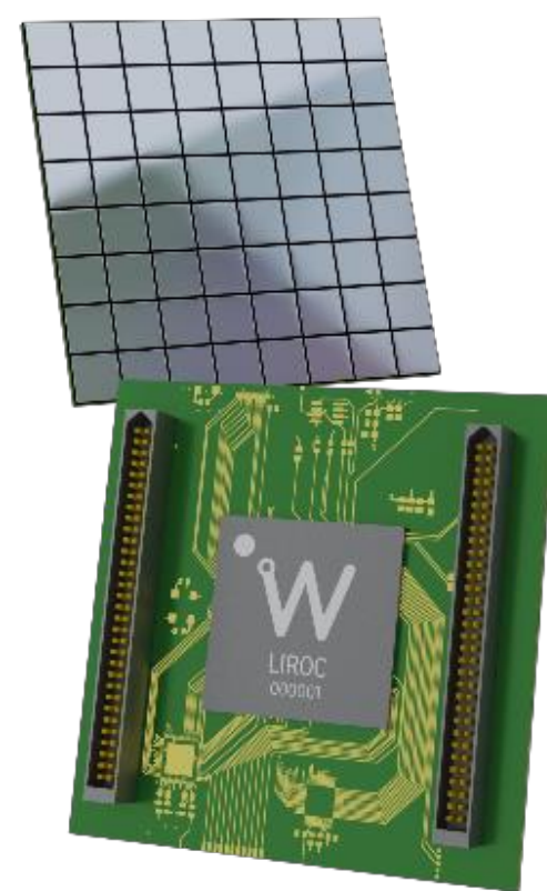
S13361-2050AE-08 by HAMAMATSU 8x8 sensors on each unit
