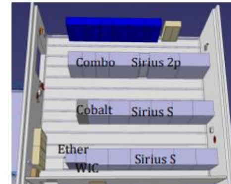
Figure 7 — Building 197/1-401: possible integration of SIRIUS converters.
