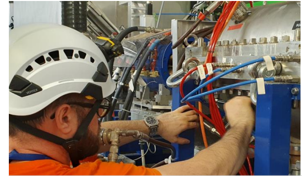
9GAP vacuum leak: tightening the bolts
