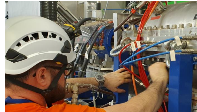
REX 9GAP vacuum leak: tightening the bolts
