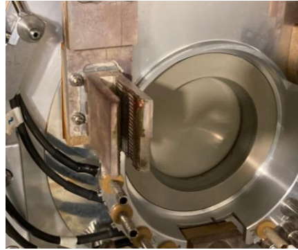
New Multicontact for main power connectors (more elastic, less friction...)
