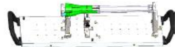
9) Install dummy staves 10) Remove from fixture 11) Test-fit into next layer
