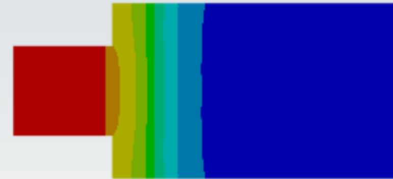
Temperature distribution of the sensor with ancillary chip, \Delta T = 27^\circ\text{C} at h_{tc} = 500 \text{ W/m}^2\text{K}
