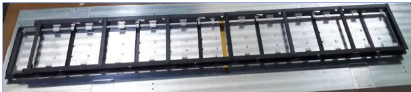
2nd Prototype Ladder – planarity < 30 microns, Sent to CERN in August 2020, validated and tested at CERN/Strasbourg, well appreciated
