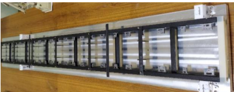
3rd Prototype Ladder – planarity < 14 microns) shipped to CERN on 14 October, 2021, Tested for performance at CERN/Strasbourg, well appreciated!
