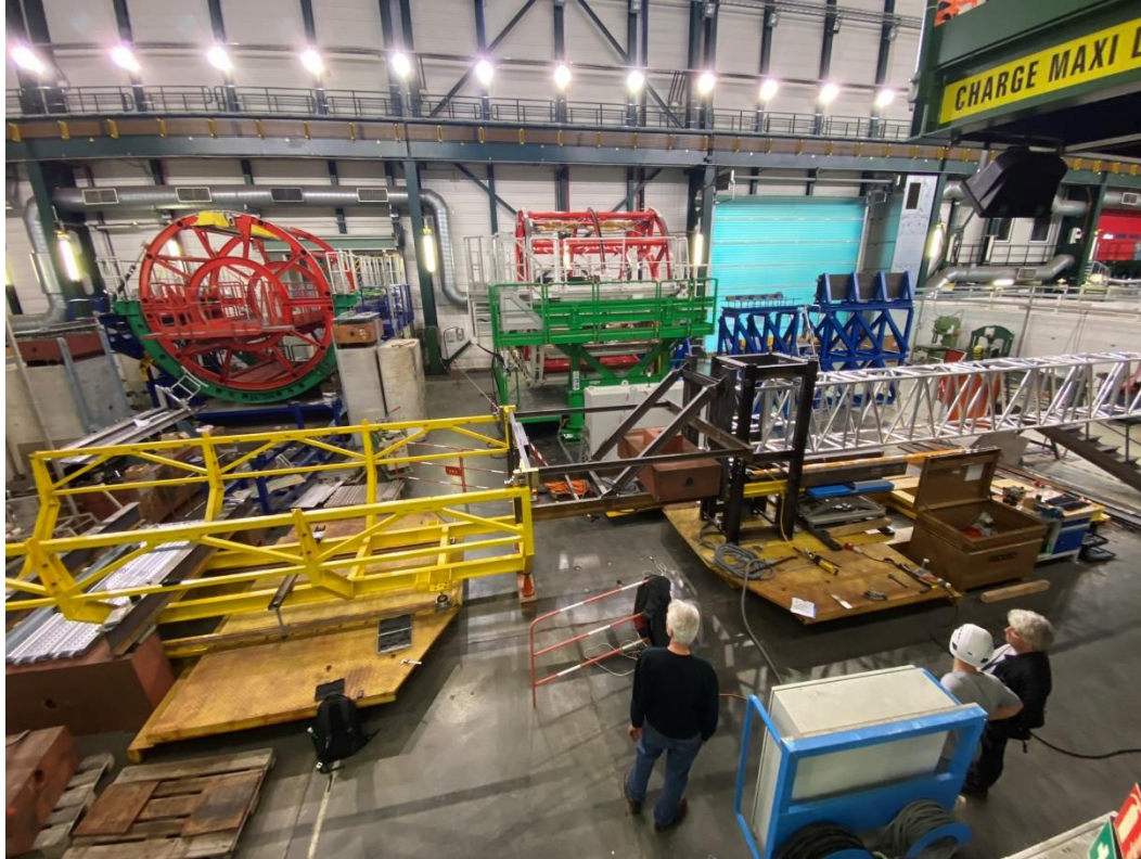
Step 3: Heaviest loading case on the vertical eiffel tower, testing the height adjustment
