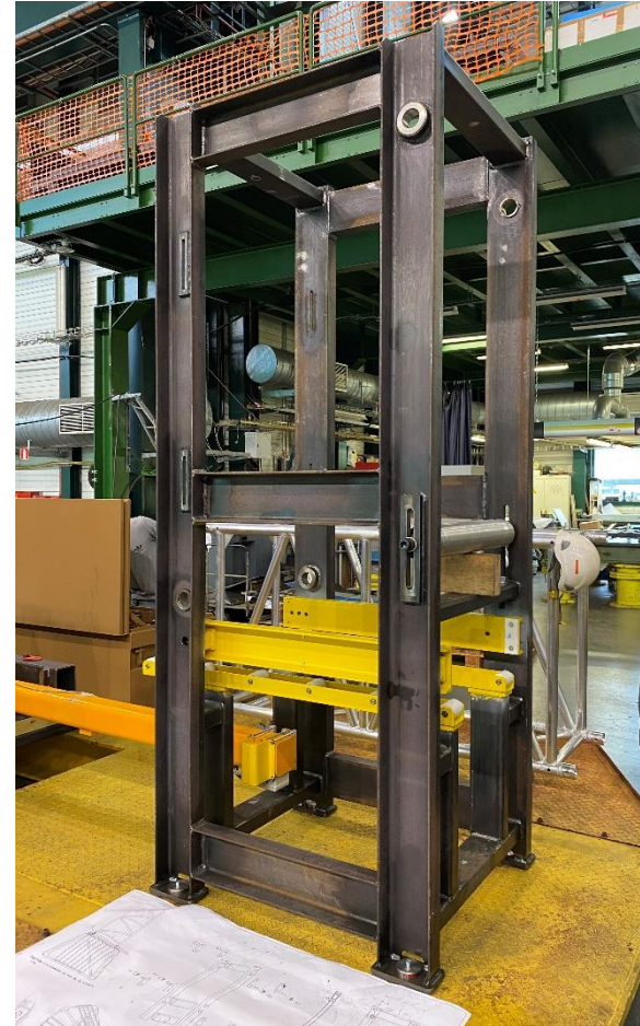
Custom design vertical eiffel tower welded from steel beams
