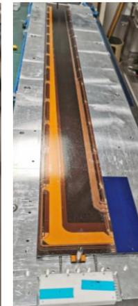
**Completed core with sacrificial edges trimmed except the ends**
