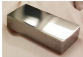
Polished block of Invar mimicking a connector
