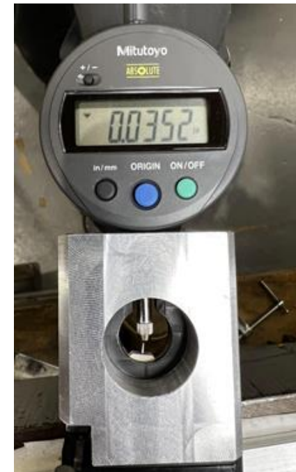
Arc gap measurement
