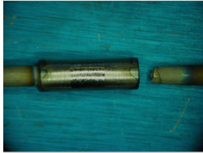
Above: Typical Tensile Test. Failure at the HAZ of the tube (right)
