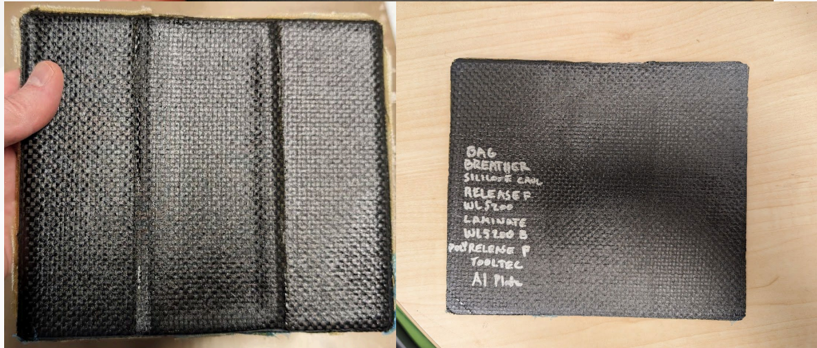
Previous Plate: Core collapsed, "F" peel ply
