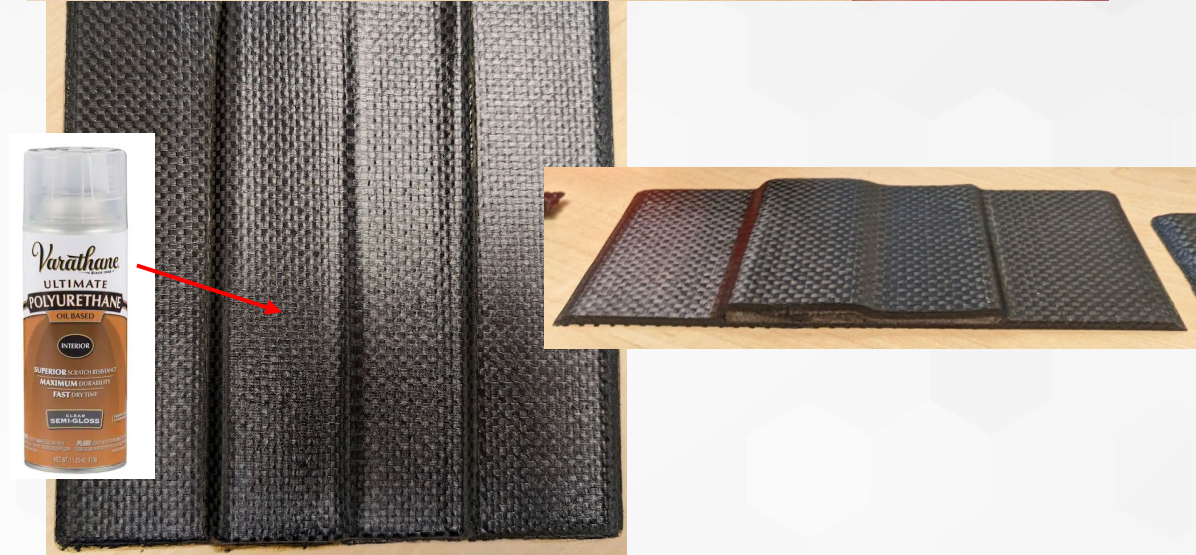
New Plate: Core held on side sealed with Polyurethane spray paint – 8 passes. "F" peel ply
