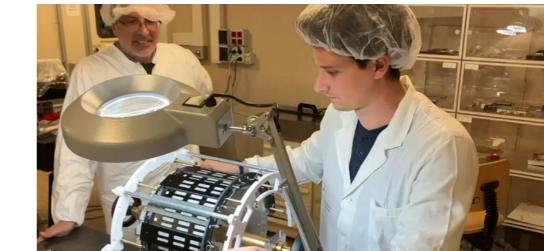
Special tool to glue the internal pillars after the extraction needed.
