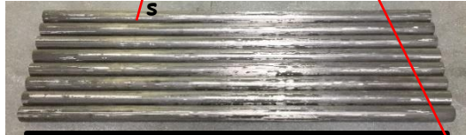
M55j/Cyanate struts roll wrapped by RWC Utah
