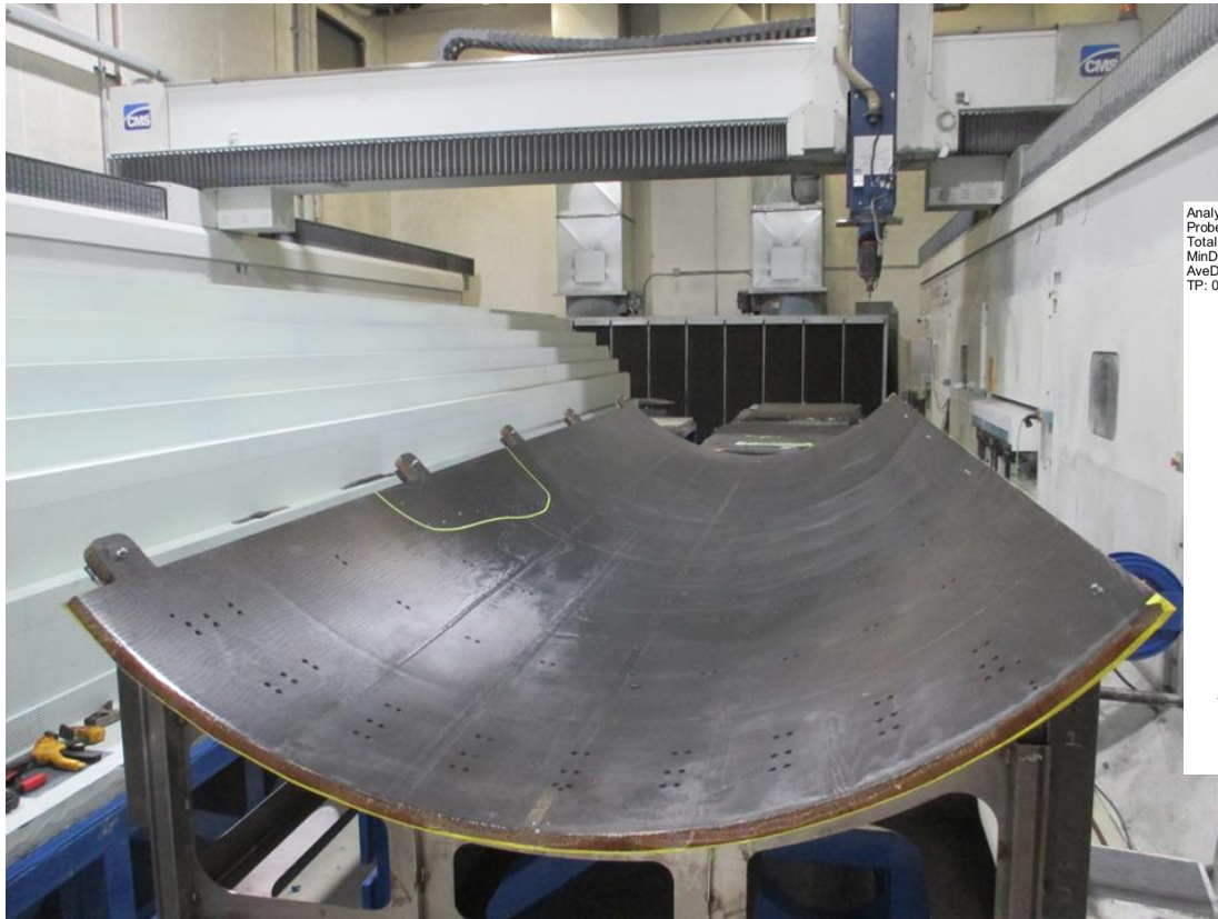
Strong Back Machining fixture holds the pre-machined qtr section to Radii during machining opp
