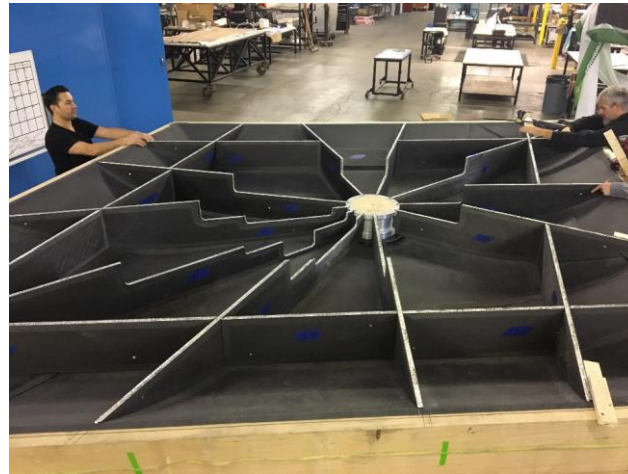
Sandwich ribs used to drive the loads to an off-center mounting hub
