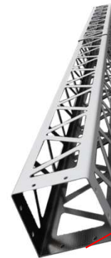
16 section expandable truss extends From each satellite
