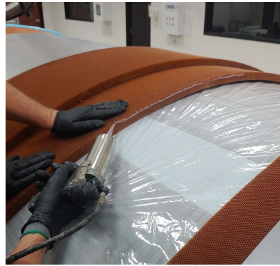
Core sheets bonded together with Arldite 2011 w phenolic micro ballons
