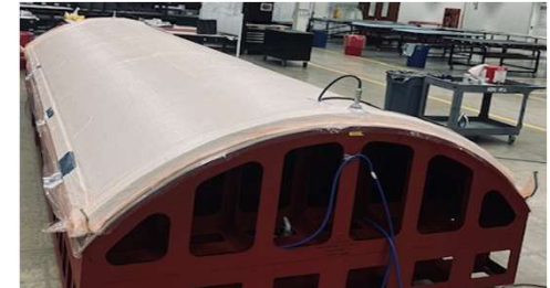
Qtr section Bagged for cure held under Vacuum for minimum of 48 hrs prior to cure
