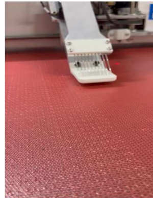
Core Perforation- poly holds vacuumed core down thru perforation process
