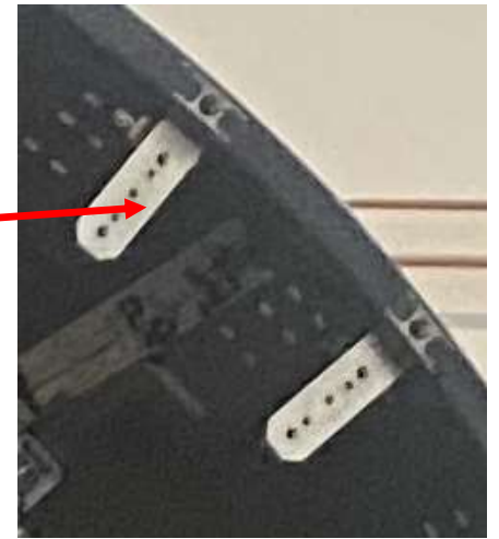
Angle Plates shown attached to inner skins by potted inserts
