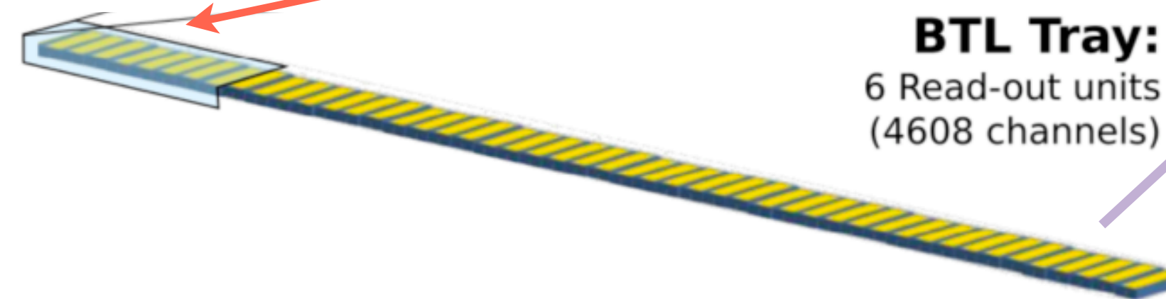
BTL detector 72 trays: 2(z) x 36(phi) 332k channels
