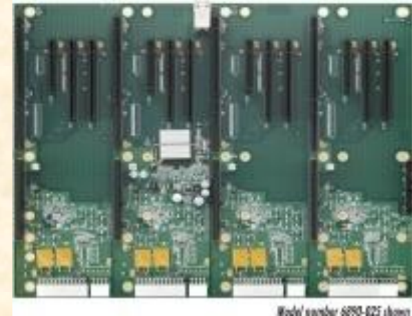
Segmented backplane with 4 SHB and 12 PCIe slots for a 19" 4U chassis
