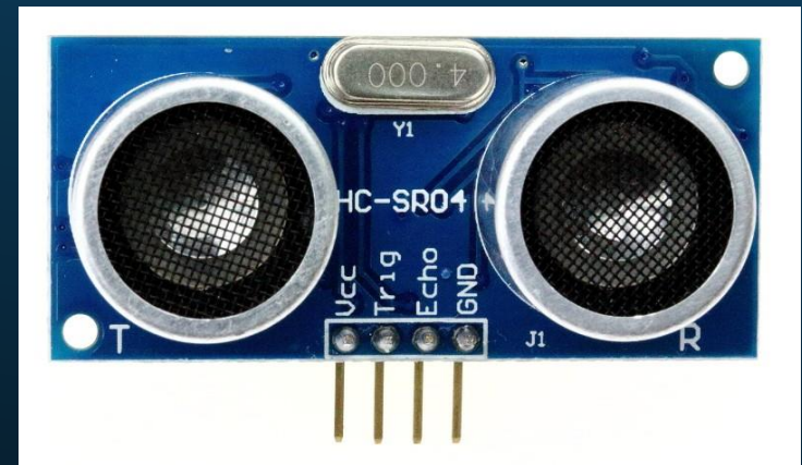
Ultrasonic distance sensor Measures distance based on the time to echo of an ultrasonic pulse.
