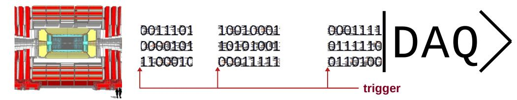
Triggerless: the detector push data at its speed and the downstream daq must keep the pace
