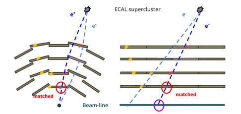
3. If a match is performed, a more precise Z position on the beamspot is determined
