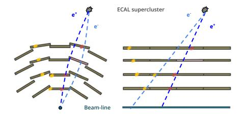
A path is propagated from the ECAL towards the beamline through the pixel detector assuming either e+ or ehypothesis
