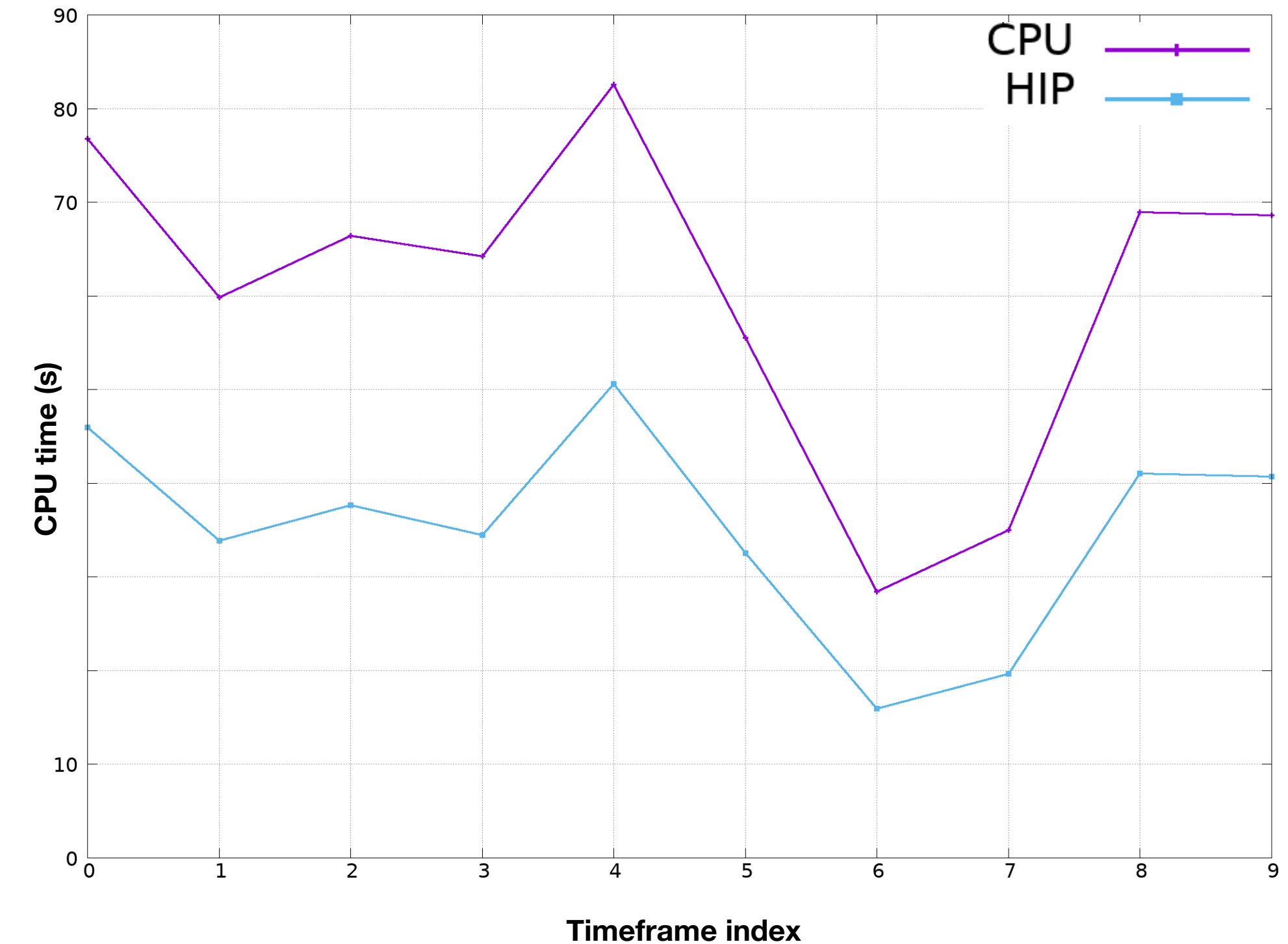
Showcase of the elapsed wall time for one thread CPU (purple) vs GPU(light blue).
