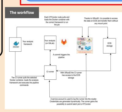
Once the jobs have been submitted to HTCondor, a loop keeps the pipeline running by checking the status of the jobs
