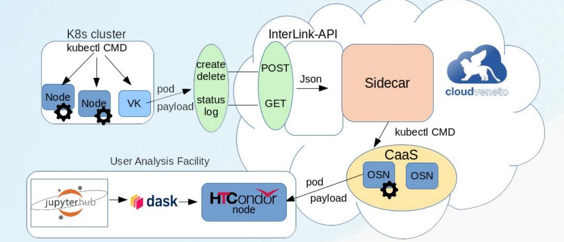
From an analysis facility users can create a dask cluster within HTCondor nodes deployed through offloading.
