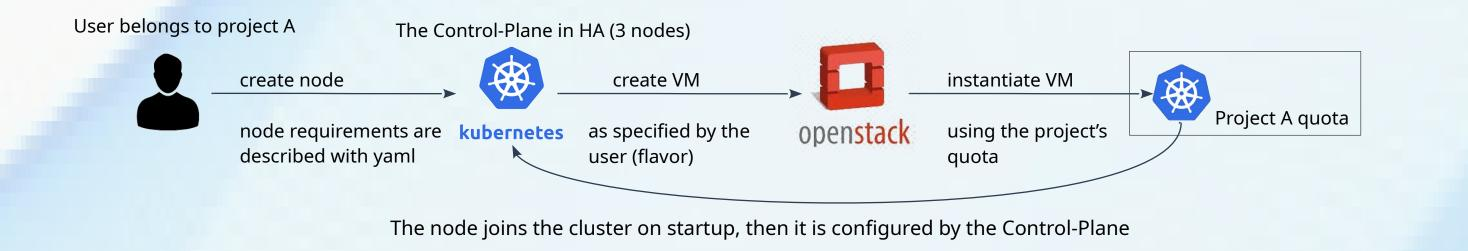
Moreover our architecture enables administrators to deploy nodes on bare-metal and dynamically scale up to handle workload spikes using cloud resources.
