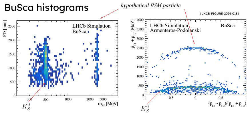
Data is stored in two 2D histograms: di-pion hypothesis mass vs flight-distance of the particle, and an Armenteros-Podolanski plot.
