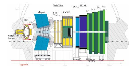
Forward spectrometer (2 <  $\eta$  < 5). 9.5 fb<sup>-1</sup> from Run 3 (until Oct 13, 2024).
