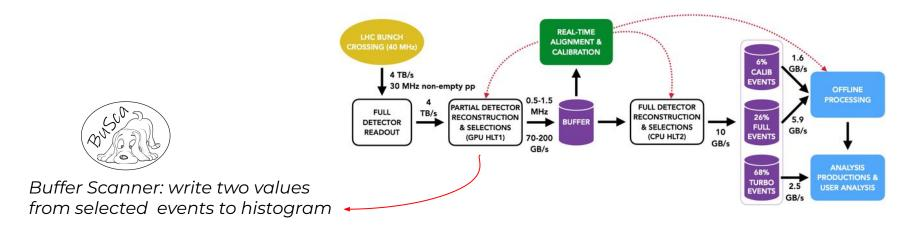
We introduce a model independent algorithm at HLT1 level. It fills 2D histograms using all available data in real time (30 MHz). It is used to guide further BSM searches. Several trigger lines are developed in this framework.
