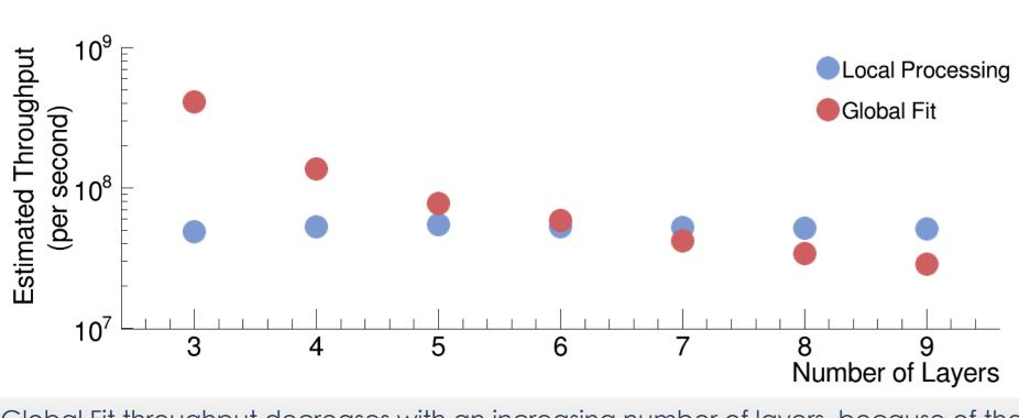
Global Fit throughput decreases with an increasing number of layers, because of the matrix inversions. Local Processing Kernel scales with the number of triplets.
