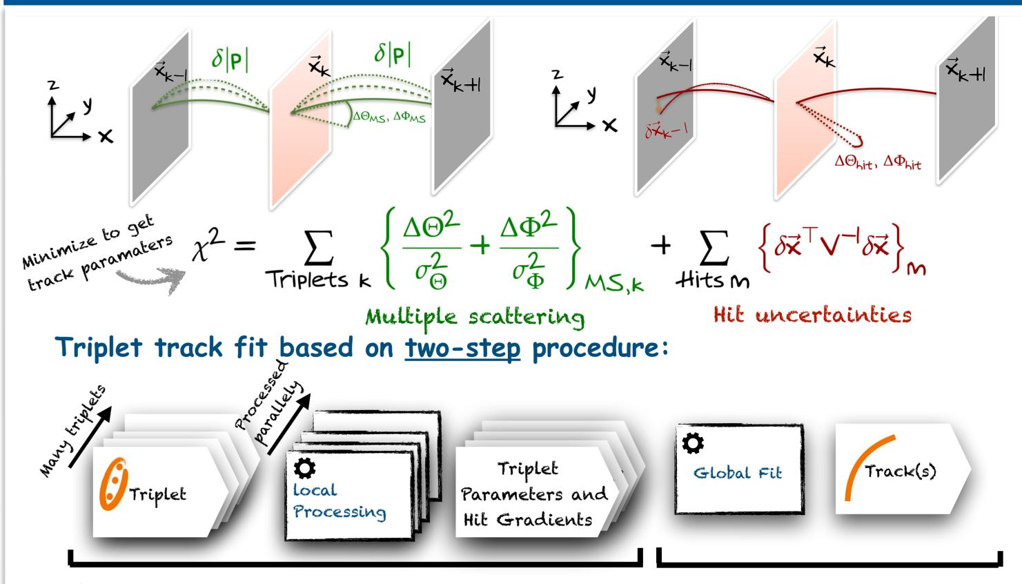
(1) Accounts for all detector-specific information, e.g., B field, material budget. Local Fit is optional for filtering. (2) Detector independent; compute track parameters from triplet parameters.
