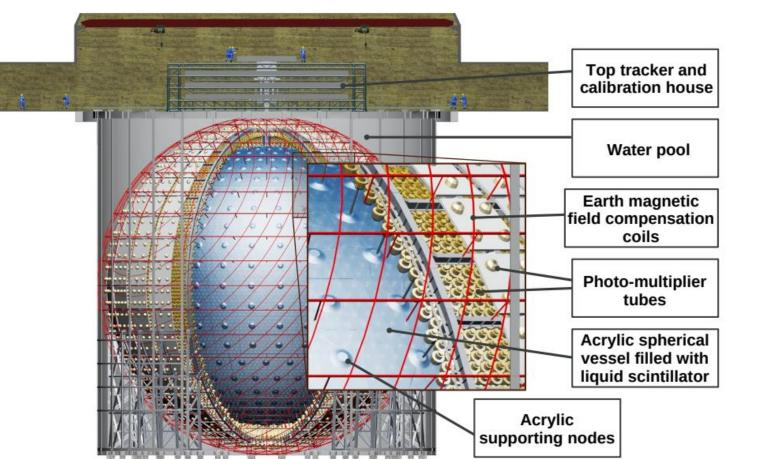
> The central detector of JUNO covered by 20000 20-inch PMTs and 25000 3-inch PMTs, electronics simulation(ElecSim) contain "hit" level of event mixing algorithm, PMT response, electronics response, trigger simulation, electronics simulation are an integral part of JUNO simulation
