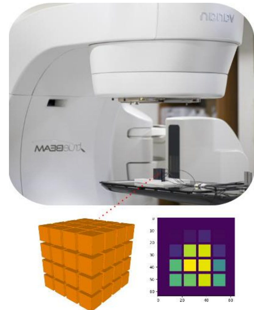
Figure 1: The experimental setup at the Linac facility of the Maria Skłodowska-Curie National Research Institute of Oncology, Krakow Branch, with a spatial dose detector phantom placed in the beam path. The phantom, featuring a 1 cm 3 active volume for measuring radiation dose distribution, is also modeled for Monte Carlo (MC) simulation [1].
