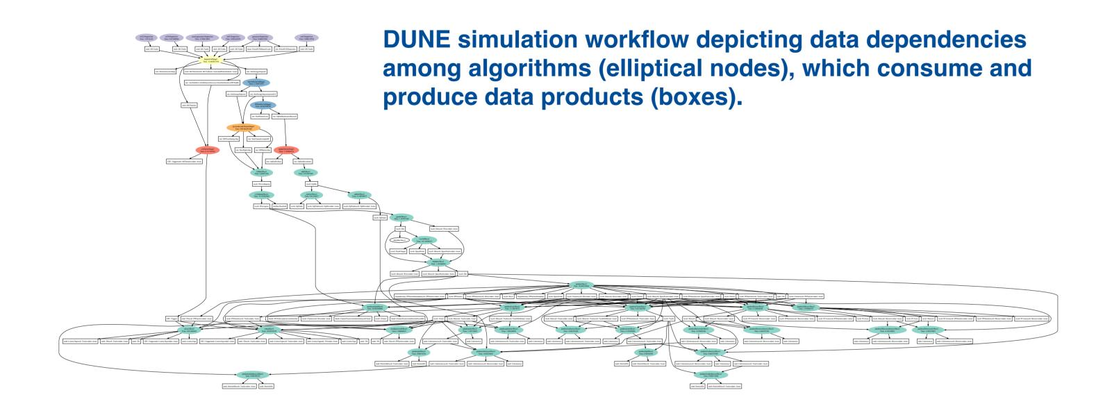
Graph-based processing approaches are not often used in HENP due to implicit dependencies between algorithms, serialization among thread-unsafe libraries, and difficulties in short-circuiting processing with filters.
