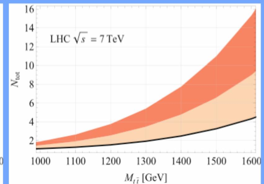
The ratio between the total and SM differential cross sections at top-pair production as a function of  $M_{t\bar{t}}$  at the Tevatron (left) and the LHC at 7 TeV (right).
