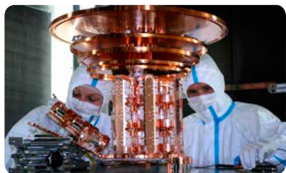
Detector Mounting at the CRESST experiment, Gran Sasso. Near the detectors, all work has to be done under clean room conditions. (Credit: CRESST)
