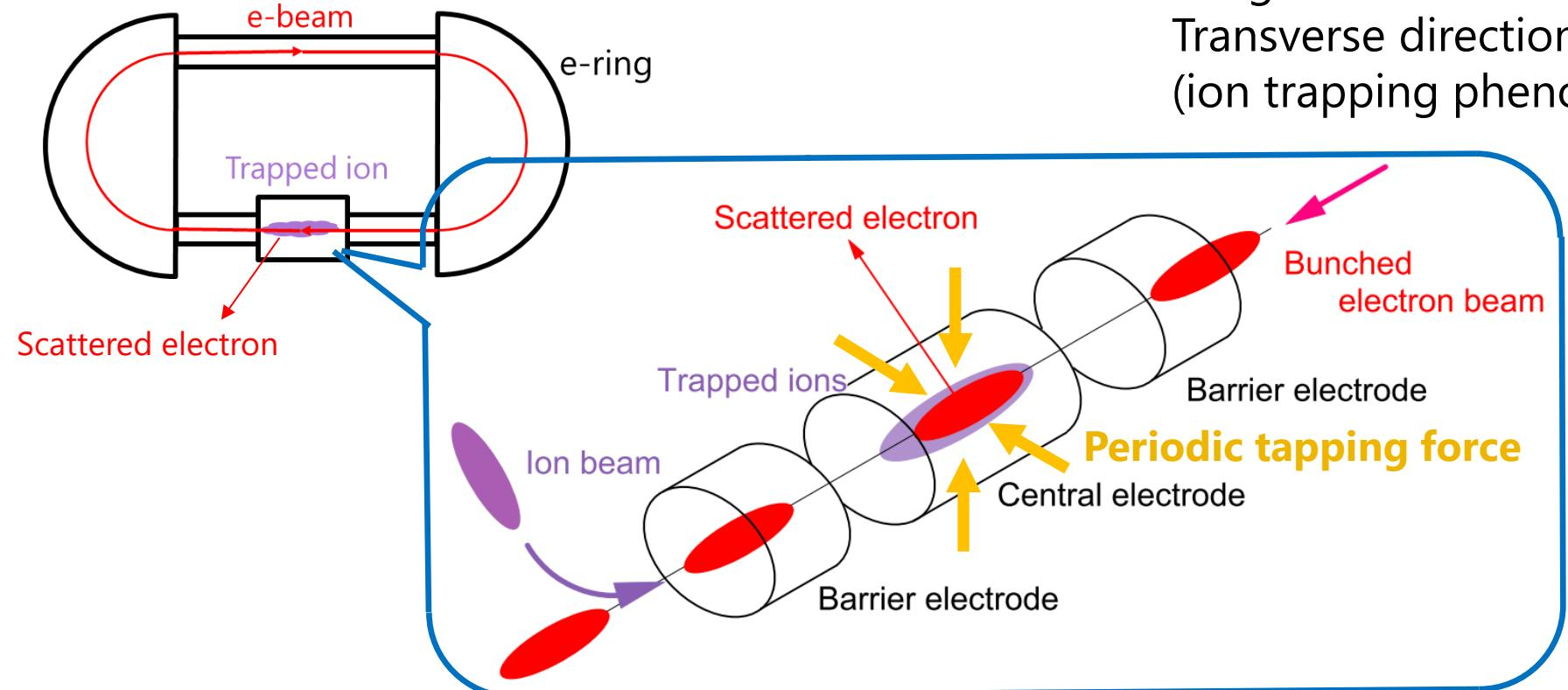
Automatic electron scattering with trapped ions
