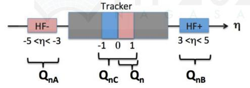
**Large** η gap  $|\Delta \eta| > 3.0$  applied to remove non-flow effects.
