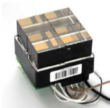
Fig. 2. MCP-PMT with coupled quartz radiator.
