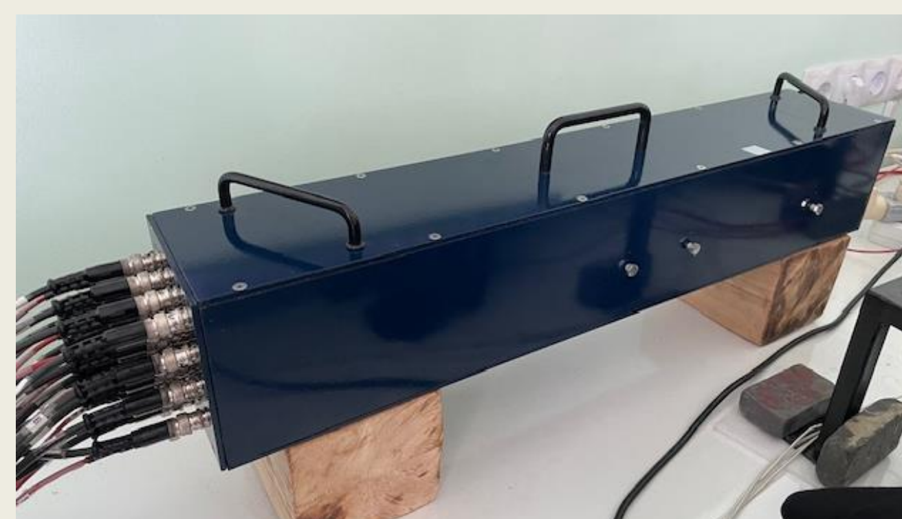
The light tight box holding the prototype assembly, and schematics of its construction and electronics for studies with cosmic rays.
