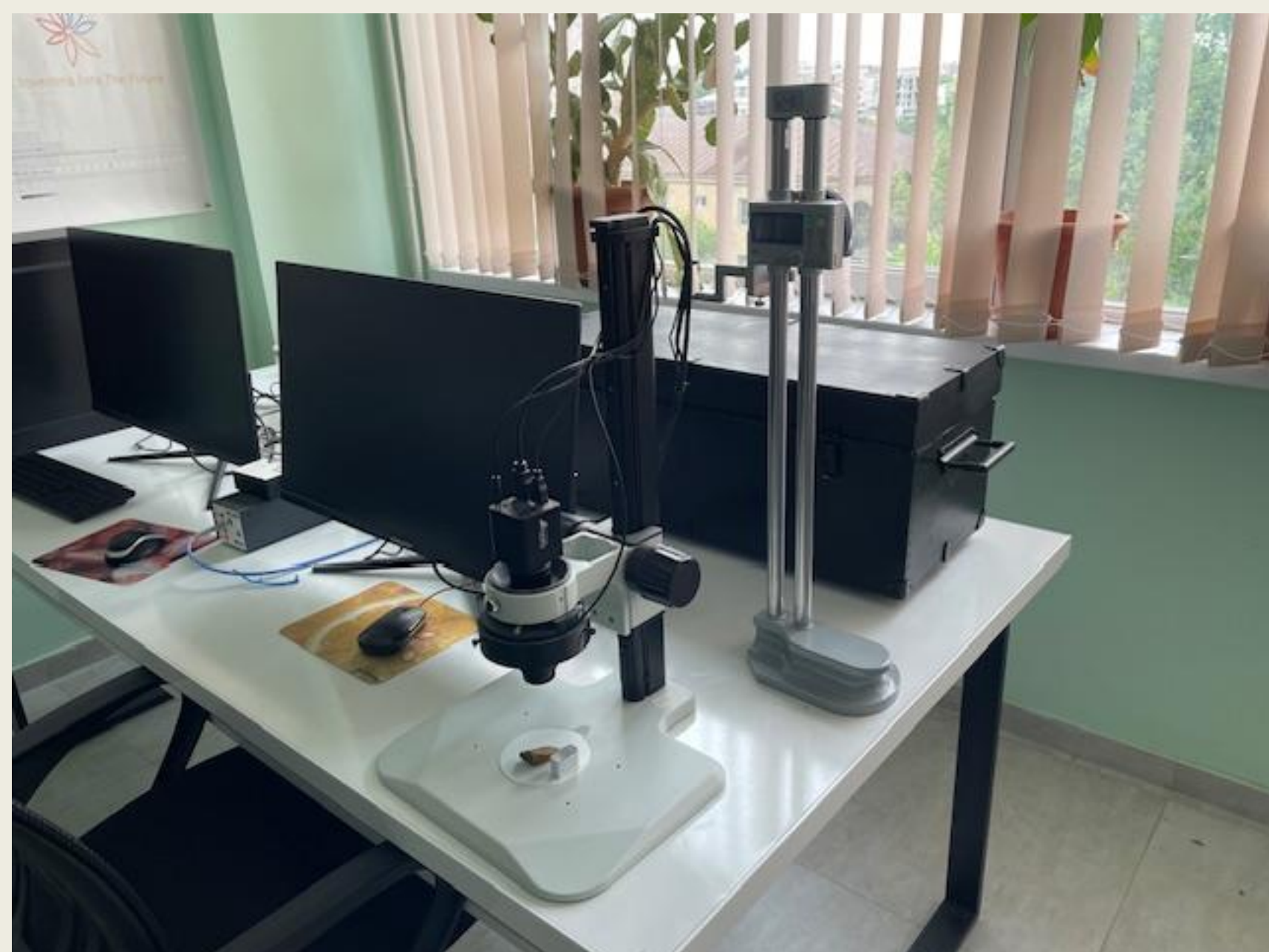
The DeltaPix digital microscope and Mitutoyo Electric Digital Height Gage sensor used in crystall quality studies.
