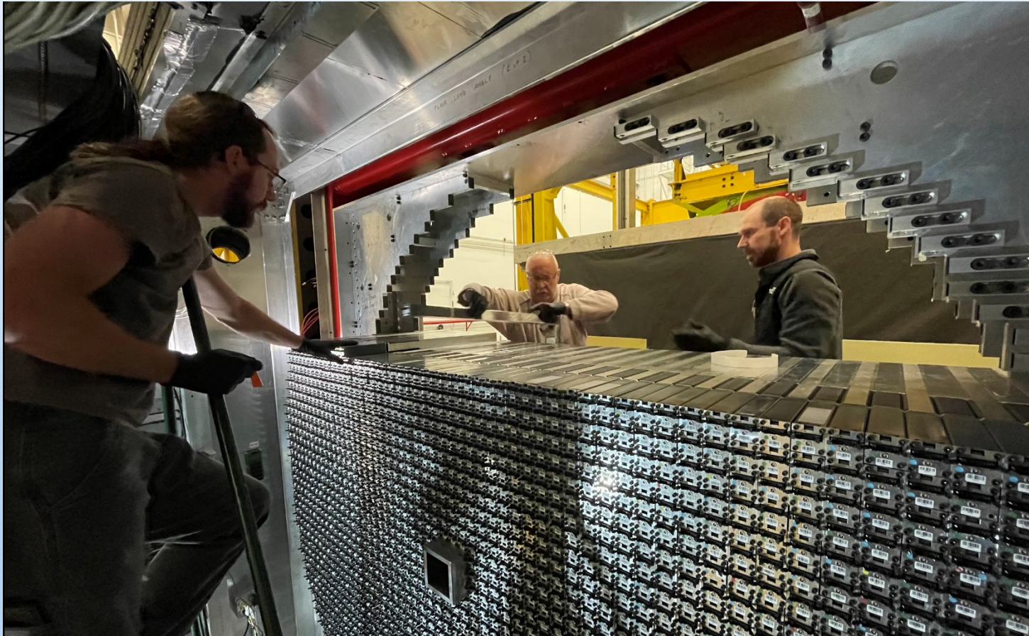
Removing lead glass modules
